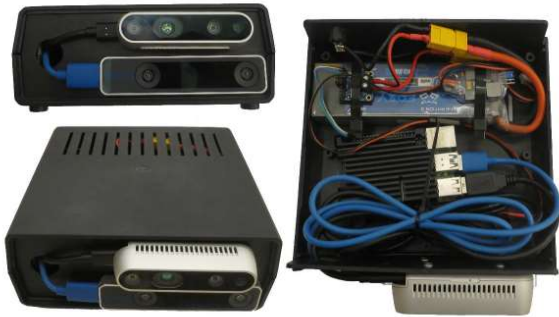
Fig. 20 The 3D handheld camera, left up) depth and tracking camera mounted on front of the handheld camera, left bottom) casing of handheld camera, right) inner components
